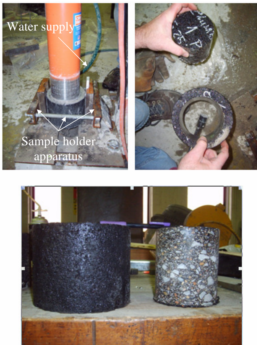
Figure 3.12 - Coring the SGC compacted HMA mixture
