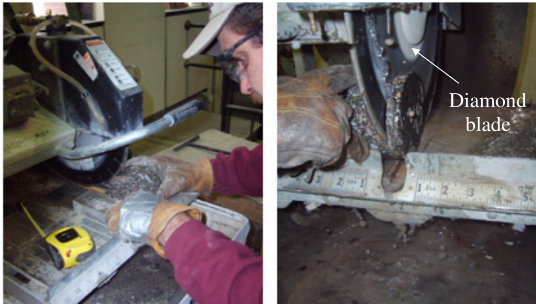
Figure 3.13 - Cutting the cored HMA sample
