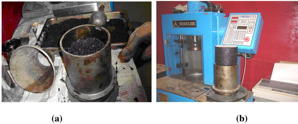
(a) (b) Figure 3.9 - Loose mixtures into the SGC mold and compacted HMA sample
